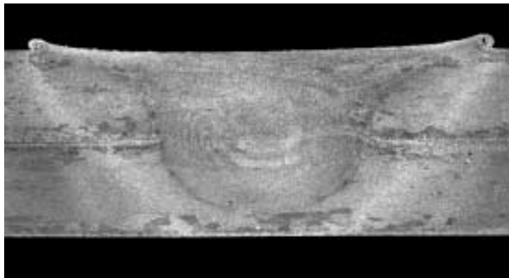
Figure 10: Lap Penetration Weld (3mm to 3 mm 6061-T6) Made with the Tower Automotive Lap Weld Tool
