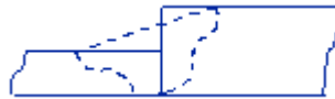
Figure 7: Friction Stir Weld of a Tailor Welded Blank from the Stepped Side
